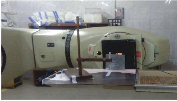
Figure 1. Test set-up for radiation attenuation
