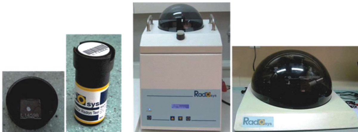
Figure 1. The CR-39 detector, diffusion chamber, RadoBath Unit, and RadoMeter microscope
