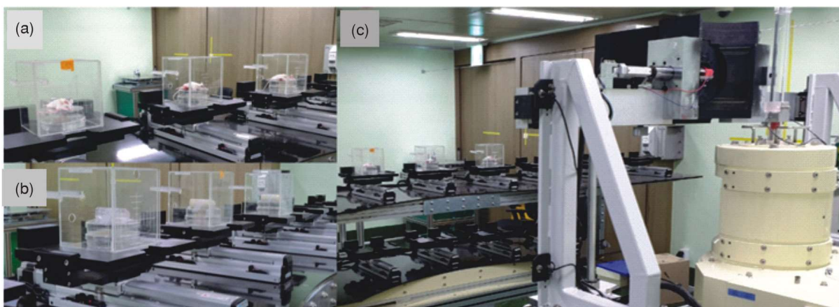
Figure 4. Experimental set-up for irradiation of laboratory mouse (a), MCNP 3-D phantom (b), and 3-D mouse phantom (c)
