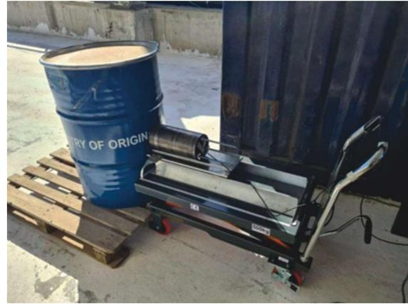
**Figure 18.** *In-situ* gamma spectrometry measurement of the Metallic drum in Configuration No. 1
