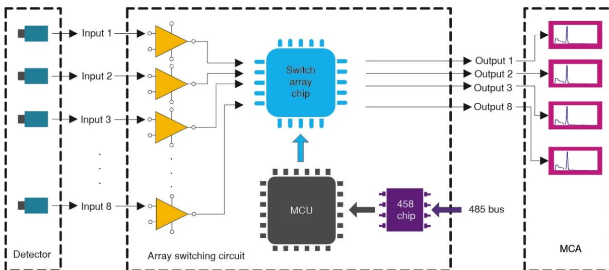
Figure 2. Multi-channel energy spectrum measurement system with the array switching circuit
