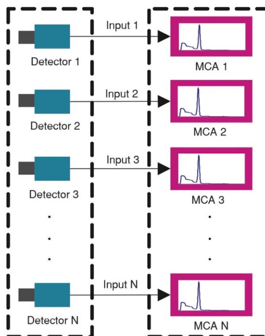
Figure 1. Multi-channel energy spectrum analyzer
