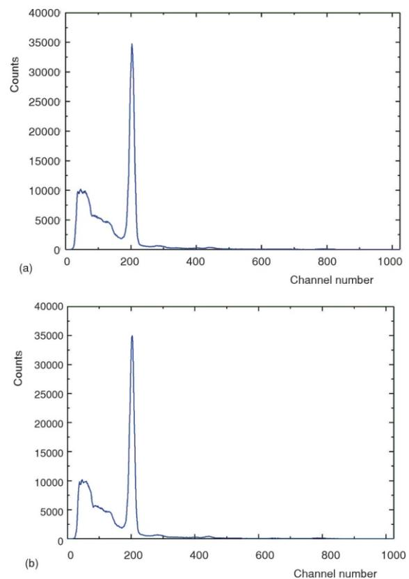
Figure 7. The energy spectrum of  $^{137}\text{Cs}$ : (a) energy spectrum obtained without the array switching circuit and (b) energy spectrum obtained with array switching circuit
