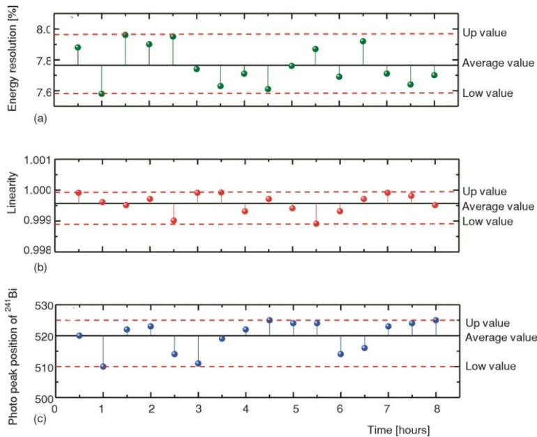
**Figure 11. Circuit reliability: (a) energy resolution, (b) linearity, and (c) photopeak position of  $^{214}\text{Bi}$**
