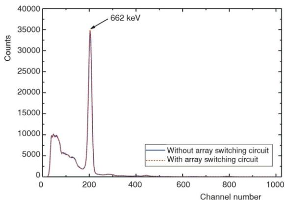
Figure 8. The energy spectrum of <sup>137</sup>Cs
