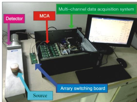
Figure 6. Experimental test system
