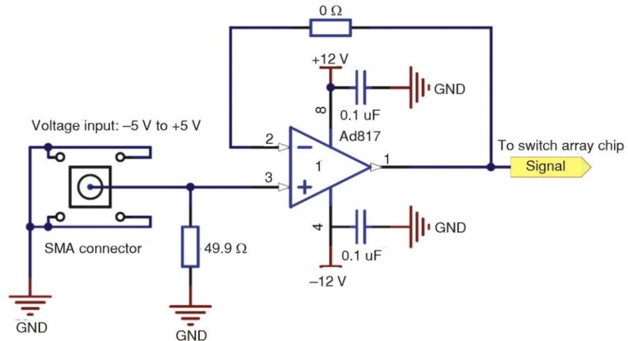
**Figure 4. Array switching circuit**
