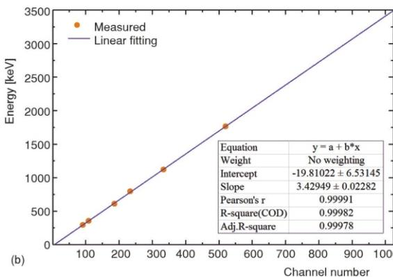
Figure 10. Energy calibration: (a) without array switching circuit and (b) with the array switching circuit
