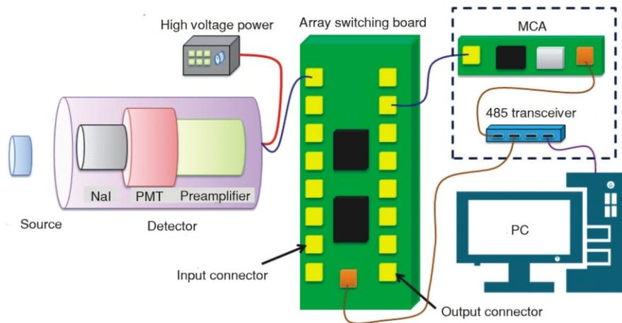
Figure 5. Experimental test system structure
