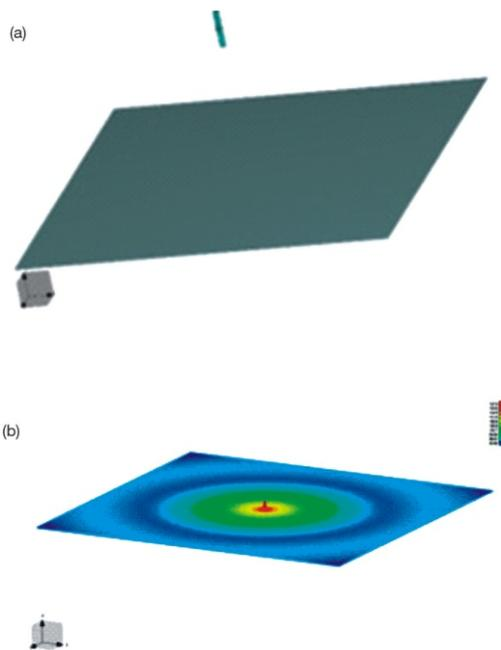
Figure 6. (a) WIPL-D model of the tubular dipole at a height of 1.29 m above PEC plane (simulated SAC) and (b) simulated near electric field distribution of tubular dipole
