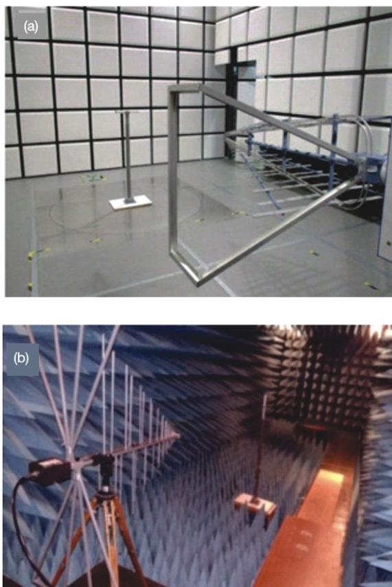
**Figure 2. Set-up of radiation emission measurement; (a) In the SAC (for case 1) and (b) In the FAC (for case 2)**
