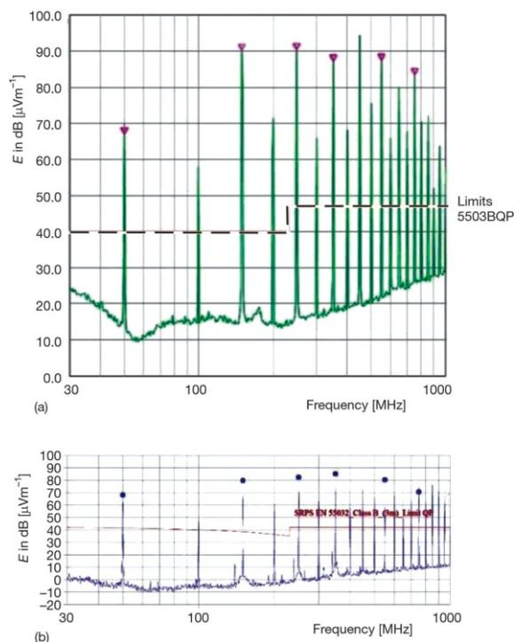
**Figure 3. Graph of measured radiation emission levels; (a) In the SAC (for case 1) and (b) In the FAC (for case 2)**
