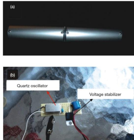
Figure 1. Tubular dipole; (a) outside and (b) inside
