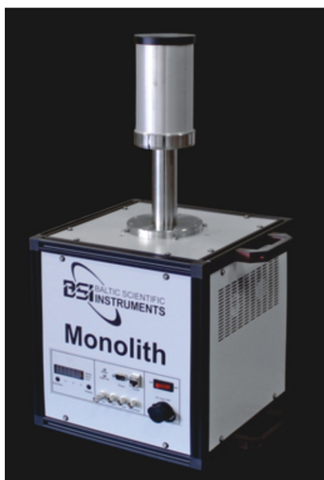
Figure 3. Photo of the HPGe detector [26] with electric machine cooling
