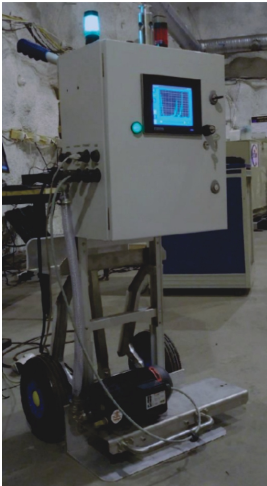
Figure 4. The mobile alpha-beta aerosol monitor
