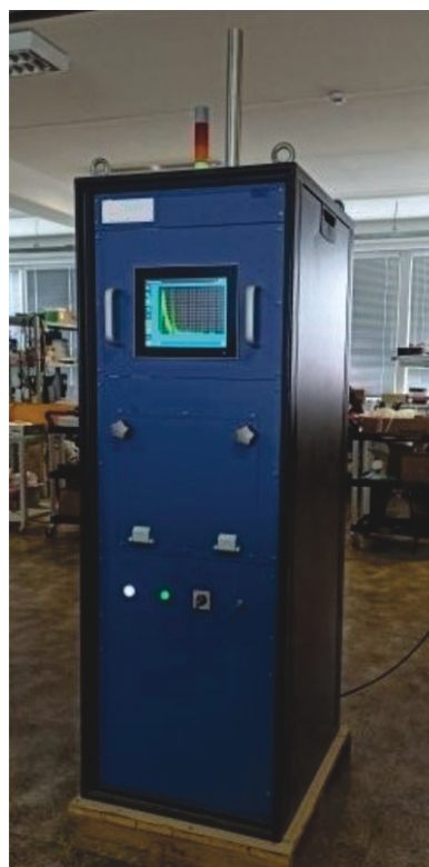
Figure 2. Photograph of the aerosol radioactivity monitor
