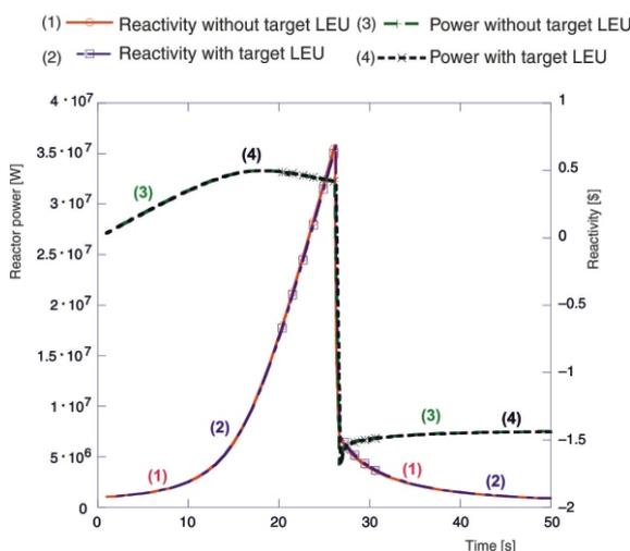
Figure 7. Net reactivity and power response at initial power 1 MW
