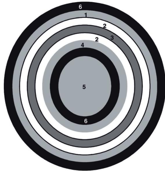
**Figure 1. Drawing for the arrangement of uranium foil target irradiation at the reactor: 1 – aluminum, 2 – nickel, 3 – uranium foil, 4 – aluminum, 5 – aluminum rod, and 6 – water**
