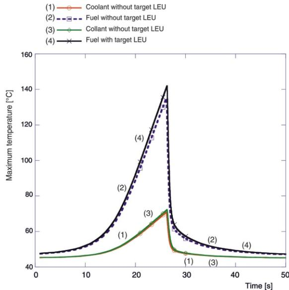
**Figure 8.** Coolant and fuel temperature during transient at initial power 1 MW
