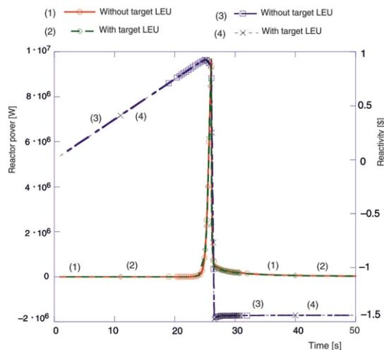
Figure 5. Net reactivity and power response at initial power 1 W
