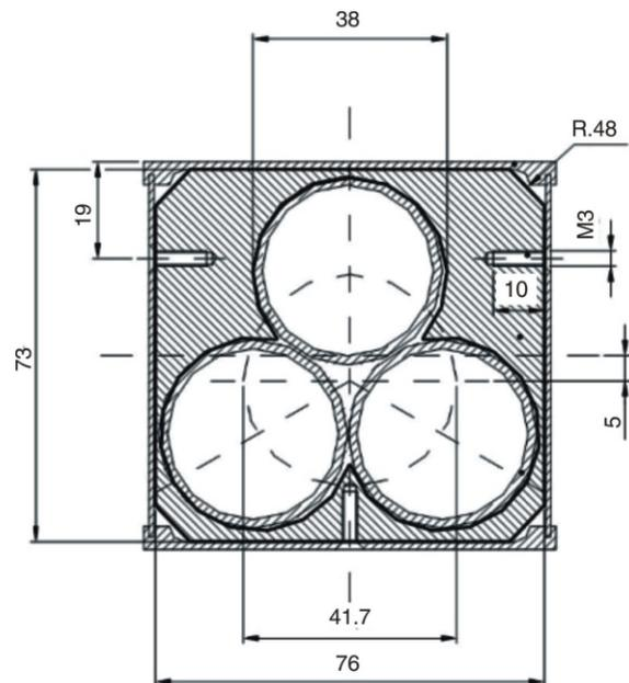
**Figure 2. Stringer for irradiation of LEU target foil (units are in mm) [8]**
