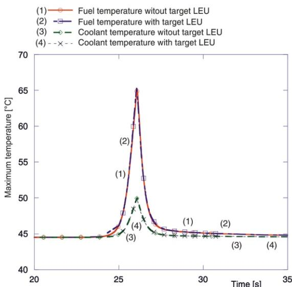
Figure 6. Coolant and fuel temperature during transient at initial power 1 W
