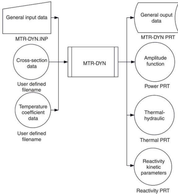
Figure 4. The MTR-DYN flow chart diagram for reactivity insertion case [14]
