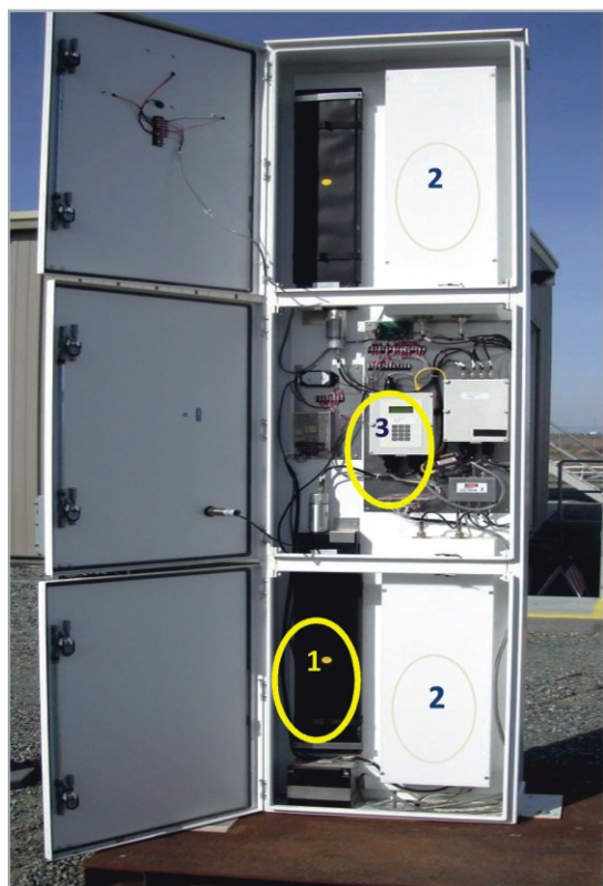
Figure 1. Pillar of RPM (model TSA PM 700 AGN) in the Greek-North Macedonia custom; 1 – gamma detectors: two scintillating detectors per pillar, 2 – neutron detectors: two in each pillar, 3 – electronics
