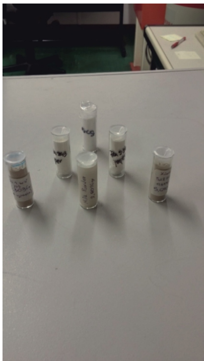
Figure 1. Volume sources produced for the calibration of the well-type detector
