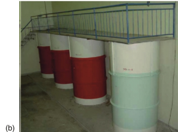
Figure 6. Standard model for measurement of coefficient of uranium-radium equilibrium; (a) standard well for logging, (b) standard well for neutron logging
