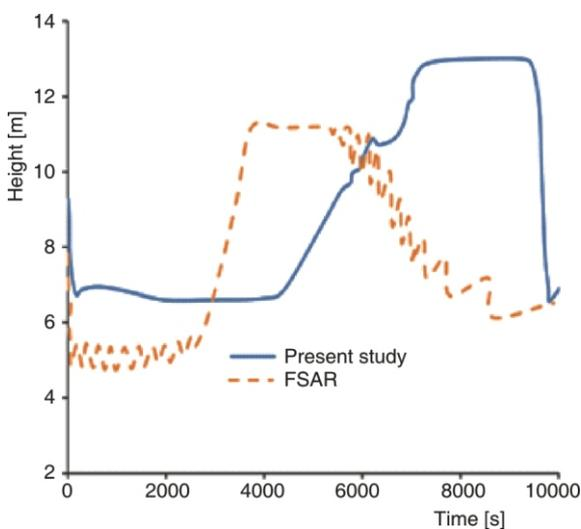
Figure 6. Water level of pressurizer
