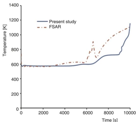
Figure 8. Fuel cladding temperature
