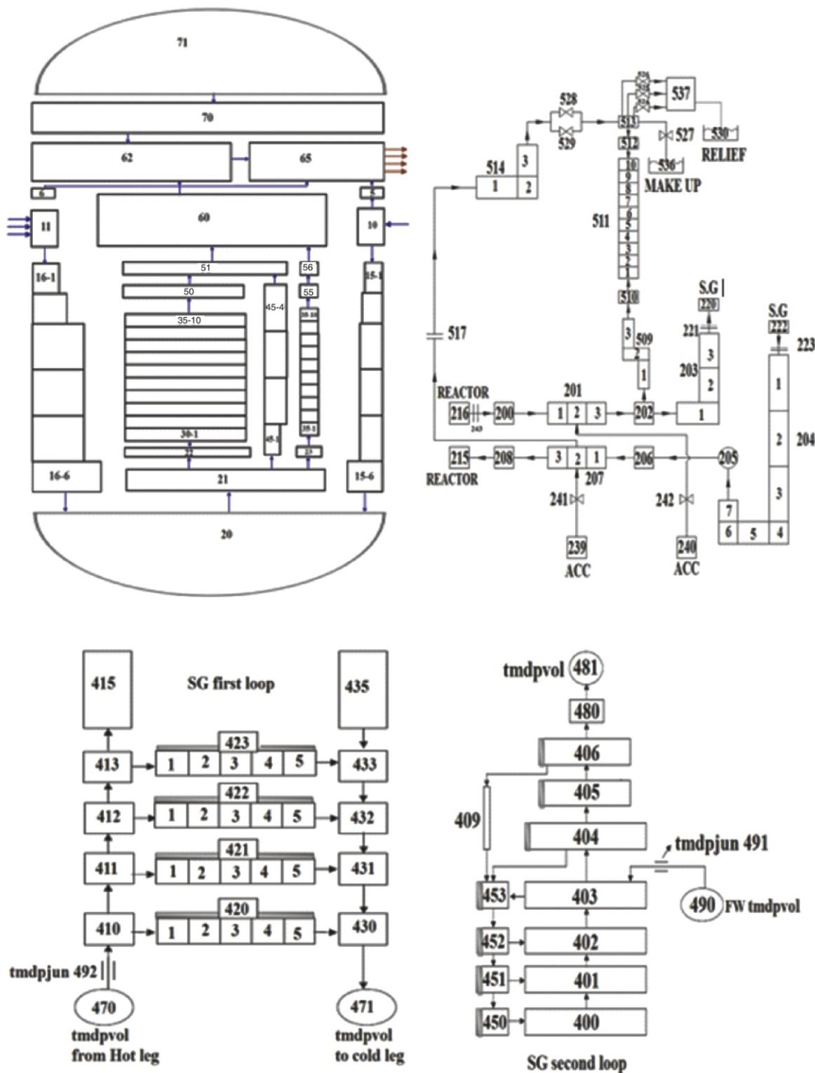
Figure 1. The VVER-1000 reactor/ Nodalization scheme
