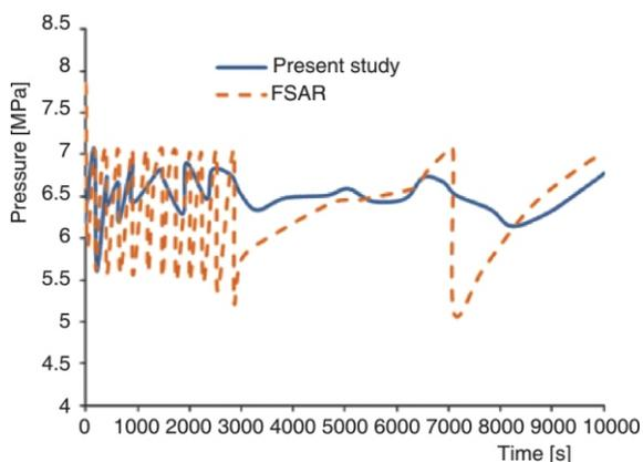
Figure 4. Secondary side pressure
