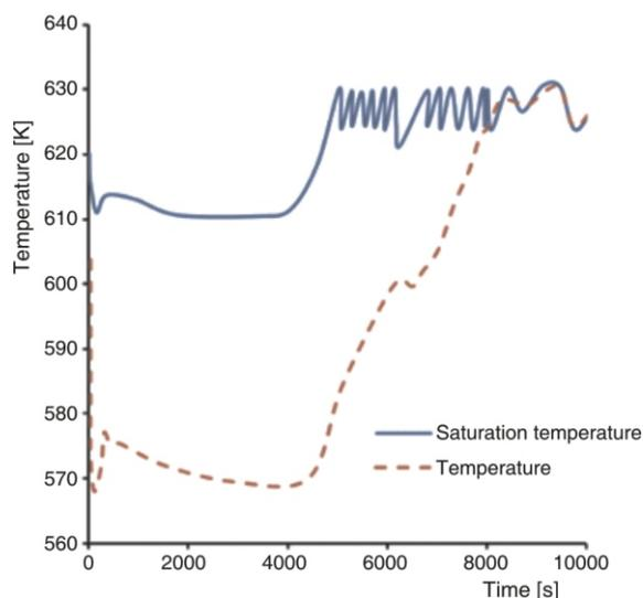
Figure 7. Temperature of hot leg of RCS and margin to the boiling temperature
