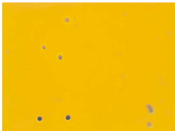
Figure 3. A magnified 1 mm × 1 mm image showing the alpha tracks that appeared on the CR-39 detector after 60 days of exposure
