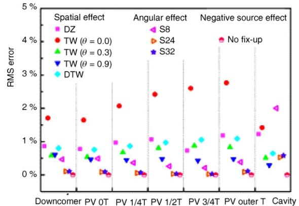
**Figure 5. Effects of  $S_N$  numeric on fast neutron fluence calculation**
