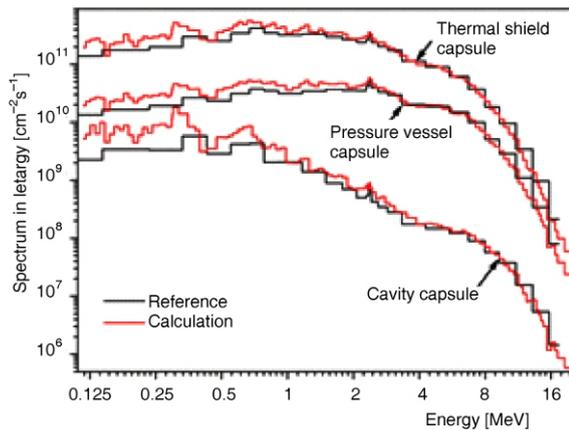
**Figure 4. Comparison of fast neutron spectrum at different capsule positions**
