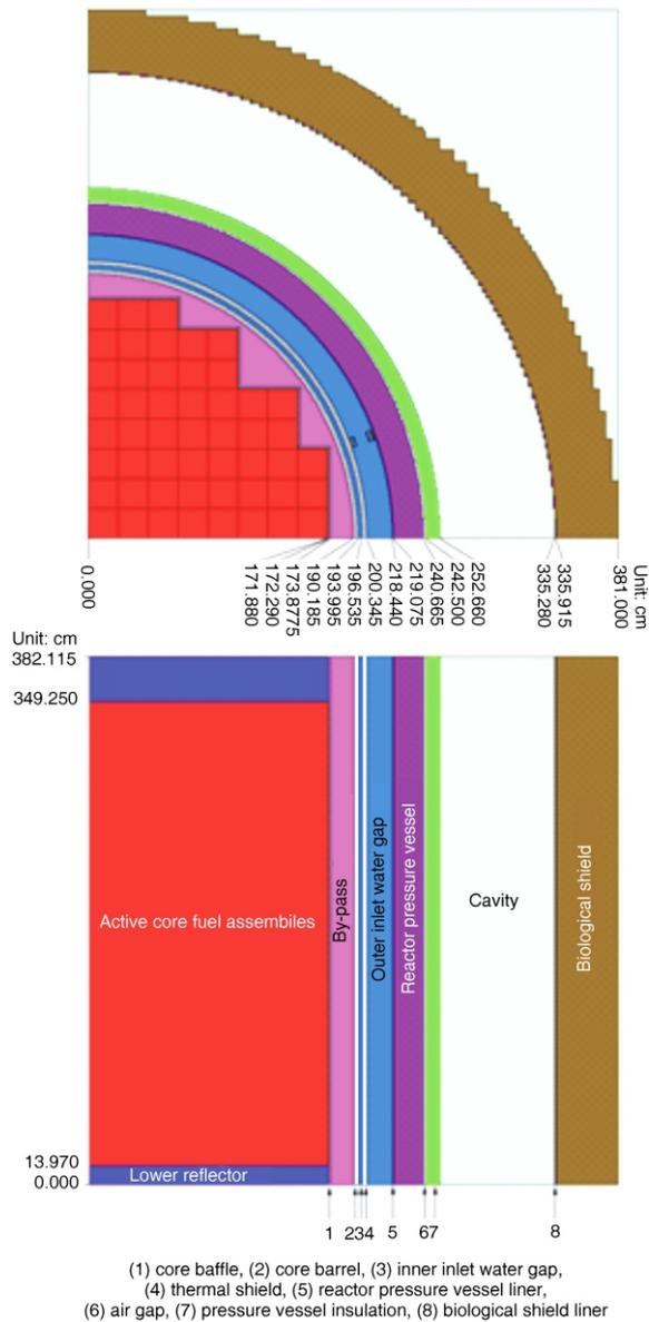
**Figure 1. Geometry configuration of the pressurized water reactor model**
