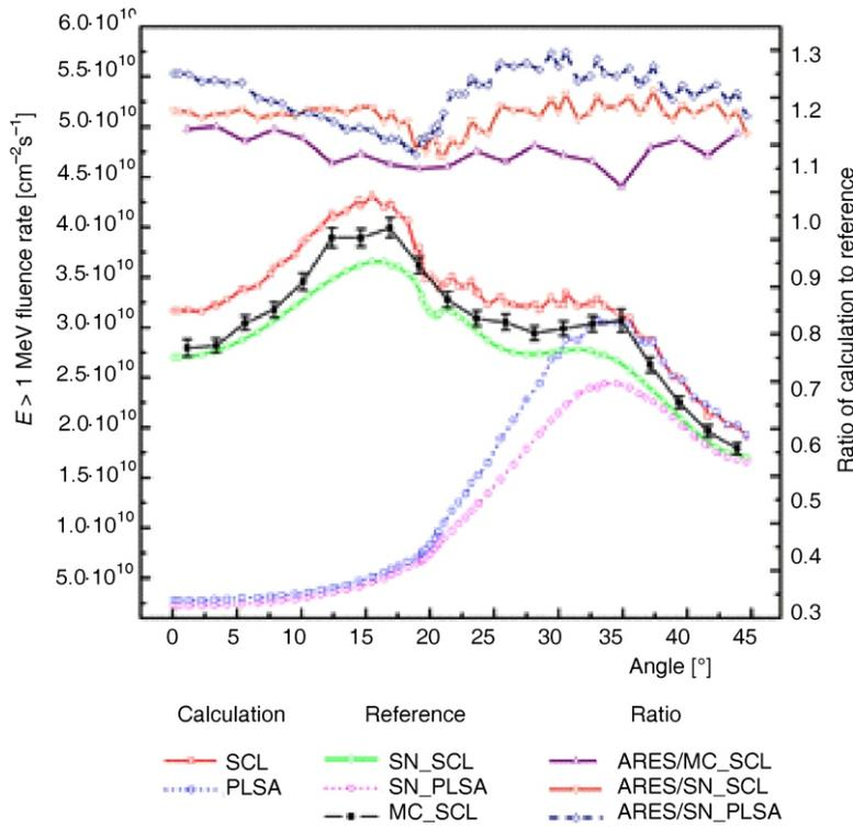
**Figure 3. Comparison of fast neutron fluence rate for model SCL/PLSA**
