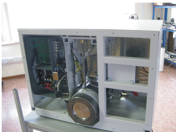
Figure 1. Spectrometric module for RPM (with opened front cover)
