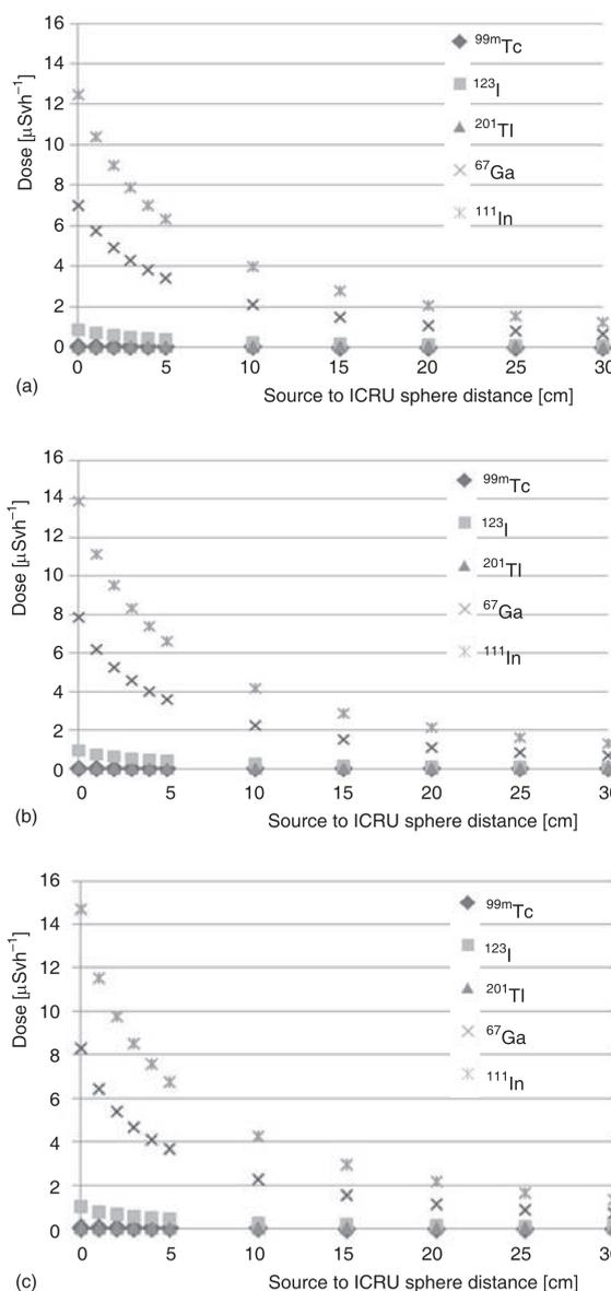
**Figure 5.** Dose according to distance between the ICRU sphere and the radiation source in using 2 mm tungsten shielding device: (a) Hp(10), (b) Hp(3), and (c) Hp(0.07)
