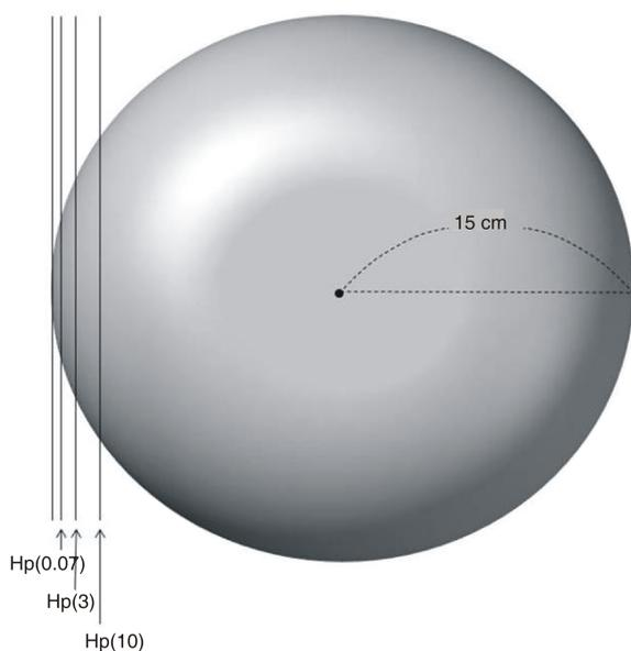
Figure 1. Simulated diagram of the ICRU sphere
