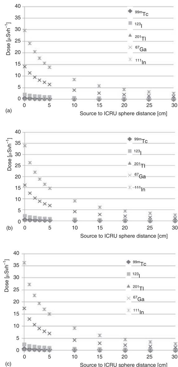
**Figure 4.** Dose according to distance between the ICRU sphere and the radiation source in using 1 mm tungsten shielding device: (a) Hp(10), (b) Hp(3), and (c) Hp(0.07)
