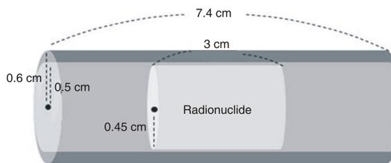
Figure 2. Simulation of radionuclide and syringe shield
