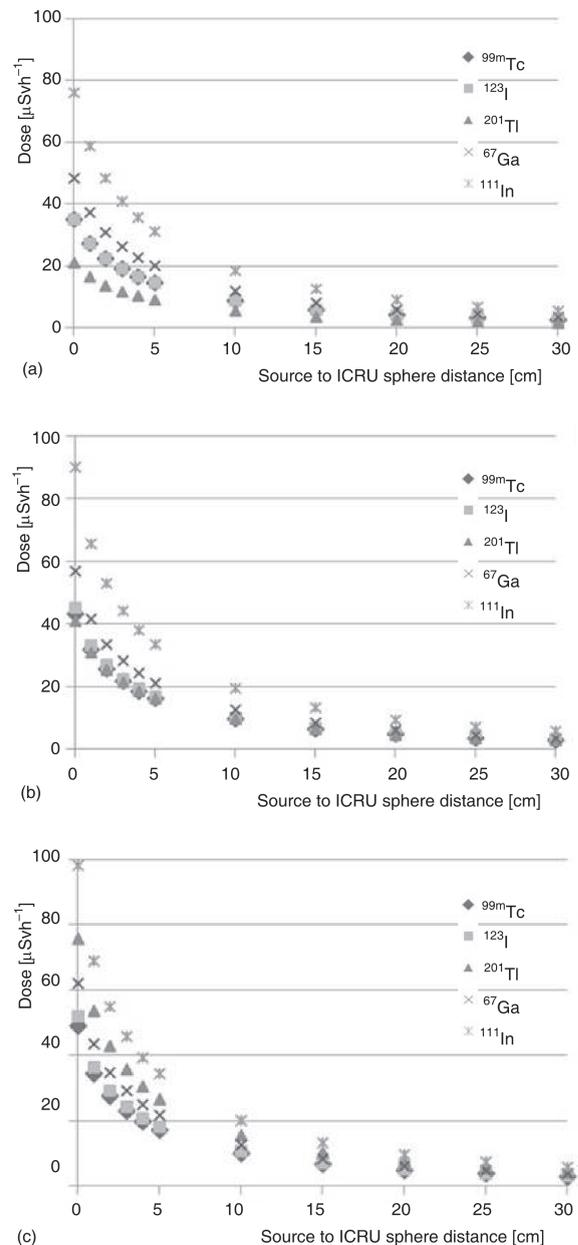
**Figure 3. Dose according to distance between the ICRU sphere and the radiation source in using no syringe shield: (a) Hp(10), (b) Hp(3), and (c) Hp(0.07)**
