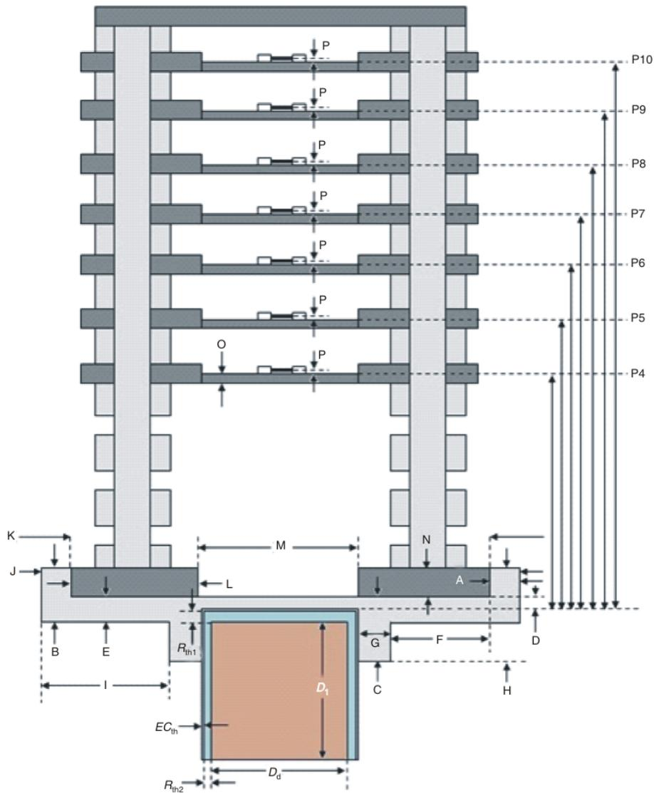
Figure 3. Schematic diagram of NaI detectors using isotropic radiating point sources measured from position P4 up to position P10
