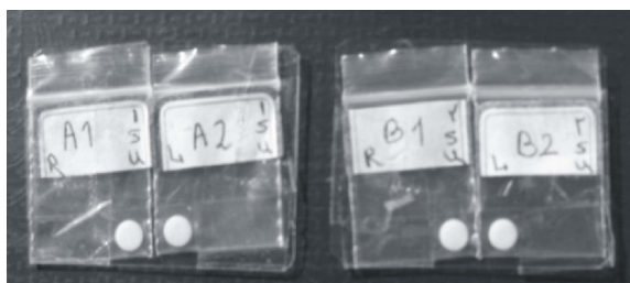
Figure 2. Used TLD packages, each package consisting of two TLD tablets
