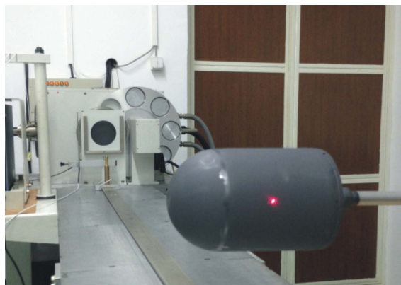
Figure 4. The ionization chamber M1000 under test with X-ray machine
