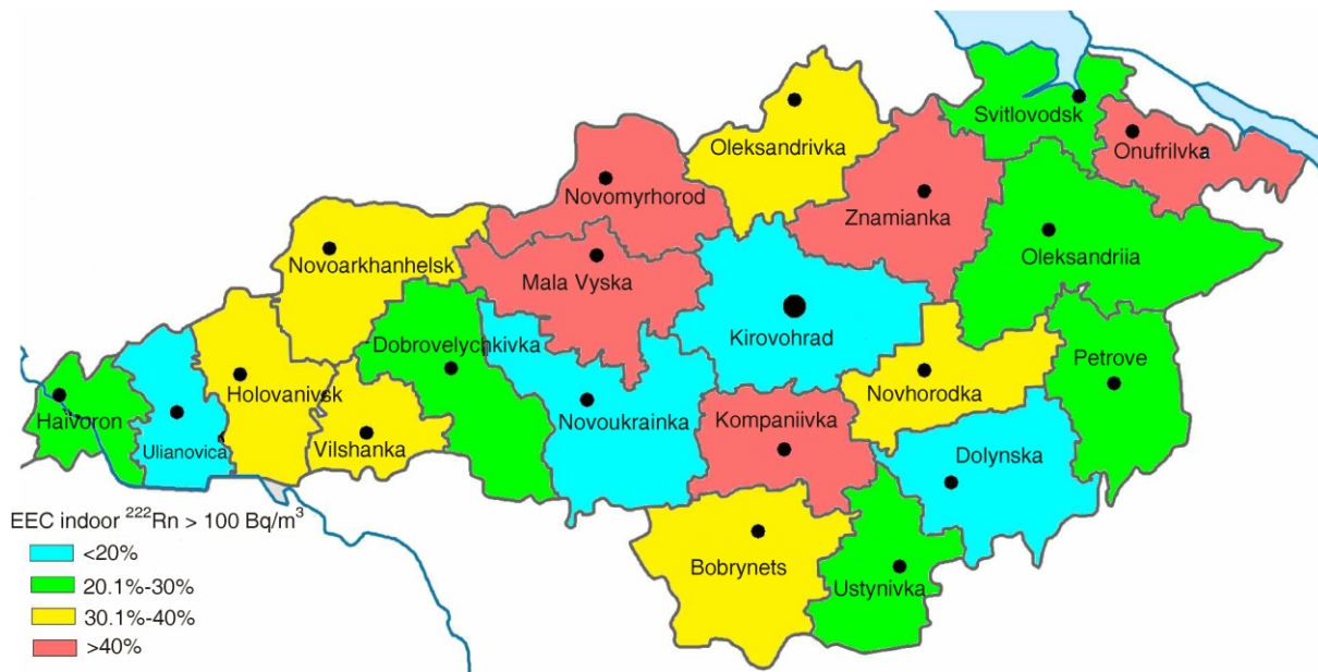
Figure 3. Ratio of buildings where the measured radon activity level exceeds 100 \text{ Bq/m}^3
