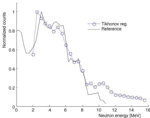
**Figure 13.** The unfolded spectrum for  $^{241}\text{AmBe}$  source obtained by the Tikhonov regularization method compared to the reference spectrum
