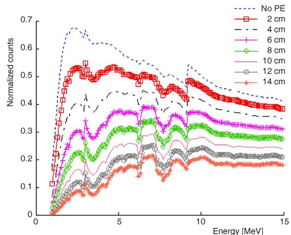
**Figure 2.** The simulated data relating the total number of counts for each energy in the range between 1 MeV and 15 MeV with step of 0.1 MeV and 8 PE layers of different thickness
