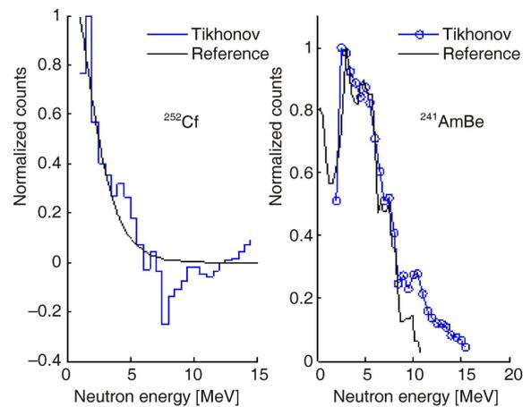
**Figure 15.** The unfolded spectrum for  $^{252}\text{Cf}$  and  $^{241}\text{AmBe}$  sources obtained by the Tikhonov regularization method compared to the reference data
