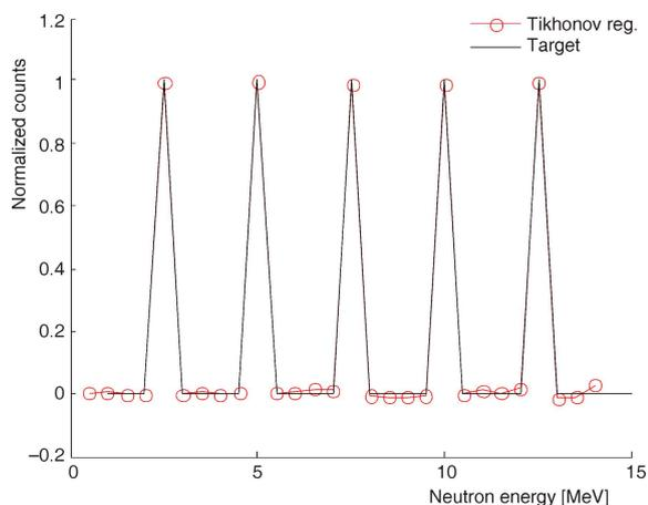
Figure 9. The unfolded results obtained by the Tikhonov regularization for a few monoenergetic neutron peaks
