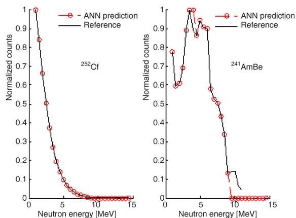
**Figure 17.** The unfolded spectra for  $^{252}\text{Cf}$  and  $^{241}\text{AmBe}$  sources obtained by the ANN approach with a Fe step of 1 cm compared to the reference data
