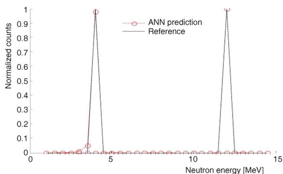
**Figure 16.** The unfolded results for the test data with a Fe step of 1 cm that have not been presented to the network before
