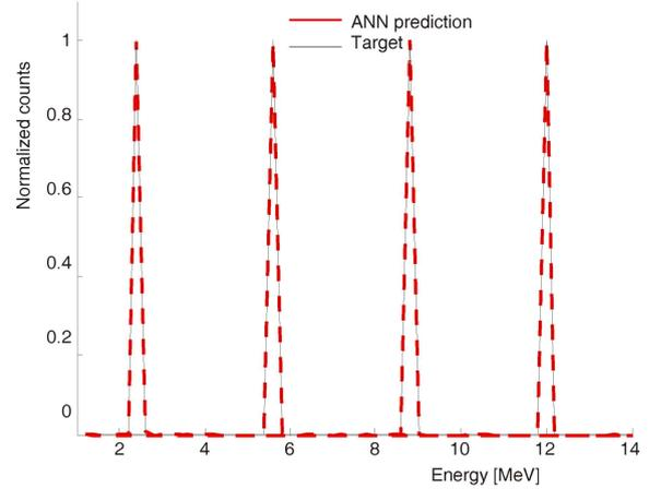
**Figure 7. The unfolded results compared with the target data for a few randomly selected test monoenergetic neutron peaks with energy step of 0.2 MeV never presented to the trained network before**
