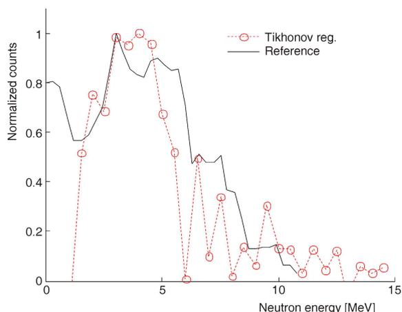
Figure 10. The unfolded spectrum by Tikhonov regularization compared to the reference  $^{241}\text{AmBe}$  spectrum (without any type of smoothing)
