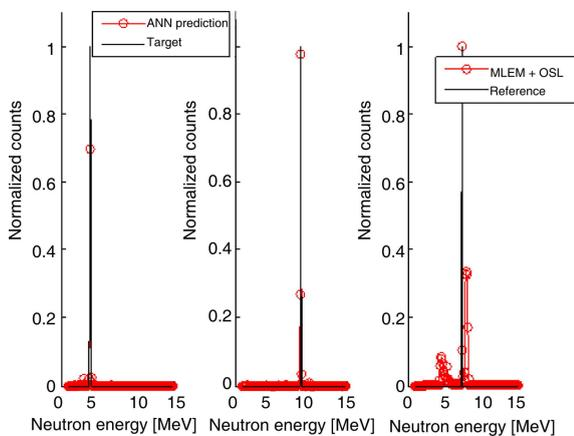
**Figure 6. The unfolded results for a few randomly selected monoenergetic neutron peaks with the energy step of 0.1 MeV obtained by the ANN approach and maximum likelihood with OSL algorithm**
