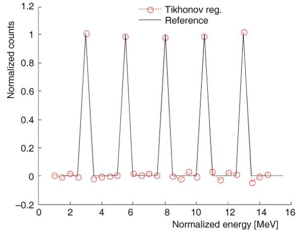
**Figure 14.** The unfolded results for a few monoenergetic neutron peaks obtained by the Tikhonov regularization method compared to the reference data
