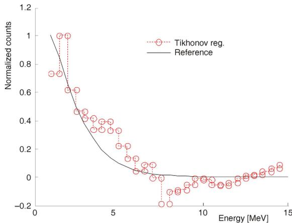
**Figure 12.** The unfolded spectrum for  $^{252}\text{Cf}$  source obtained by the Tikhonov regularization method compared to the reference data
