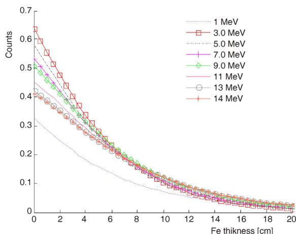
**Figure 5.** The attenuation of neutrons with different energies through Fe layers of various thickness
