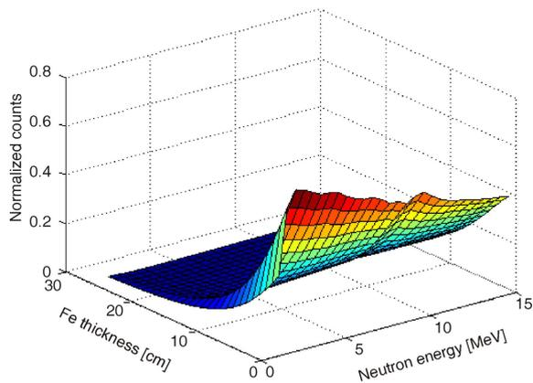
**Figure 3.** The 3-D representation of the spectrometer response matrix for the monoenergetic neutron sources between 1 and 15 MeV with energy step of 0.5 MeV and 40 Fe layers with a step of 0.5 cm between 0 and 20 cm
