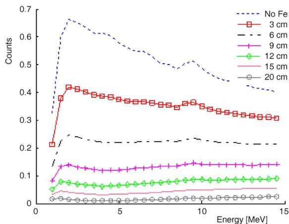
**Figure 4.** The simulated data relating the total number of counts for each energy in the range between 1 MeV and 15 MeV with step of 0.5 MeV and 40 Fe layers of different thickness with a step of 0.5 cm
