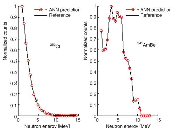
**Figure 19.** The unfolded spectra of  $^{252}\text{Cf}$  and  $^{241}\text{AmBe}$  sources obtained by the ANN approach with a Fe step of 0.5 cm compared to the reference data
