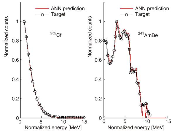
**Figure 8. The unfolded results for  $^{252}\text{Cf}$  and  $^{241}\text{AmBe}$  neutron sources obtained for the trained data with energy step of 0.2 MeV**
