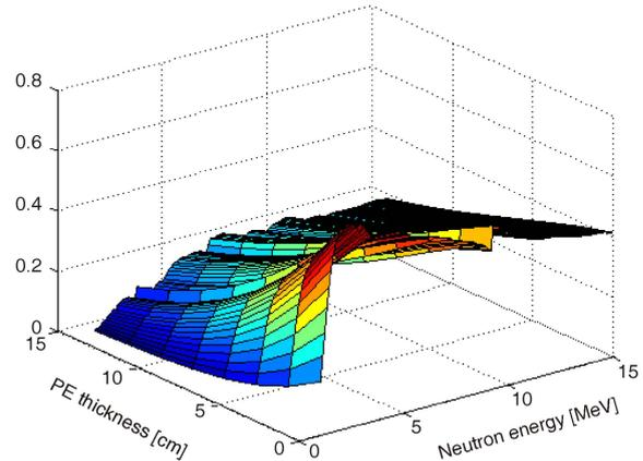
**Figure 1.** The 3-D representation of the spectrometer response matrix for the monoenergetic neutron sources between 1 and 15 MeV with energy step of 0.1 MeV and 8 PE layers with thickness of 2 cm between 0 and 16 cm
