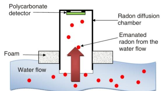
**Figure 2. Passive measurement method of the dissolved radon in water. The radon emanates from the water into a floating diffusion chamber and then starts to decay. The produced alpha particles may affect the polycarbonate on the SSNTD**
