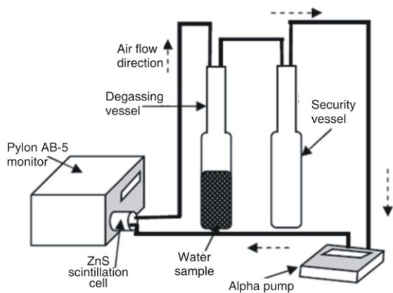
**Figure 3. Active measurement method of the dissolved radon in water. The radon emanates from the water sample into a degassing vessel and then flows into a scintillation ZnS cell via an air pump. The Pylon monitor then counts the emitted alpha particles**
