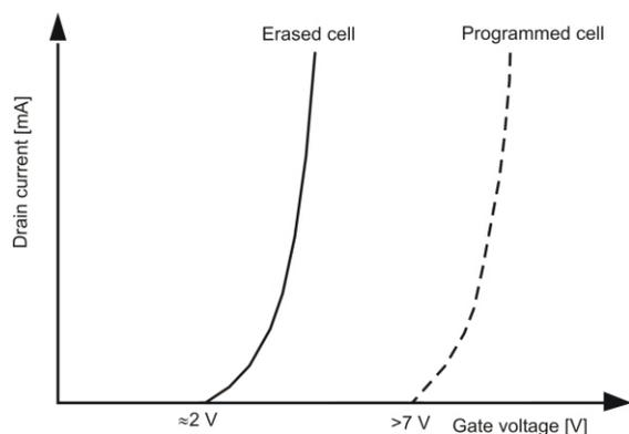
Figure 2. Flash cell's current-voltage characteristic (drain current vs. gate voltage) in the erased and programmed state
