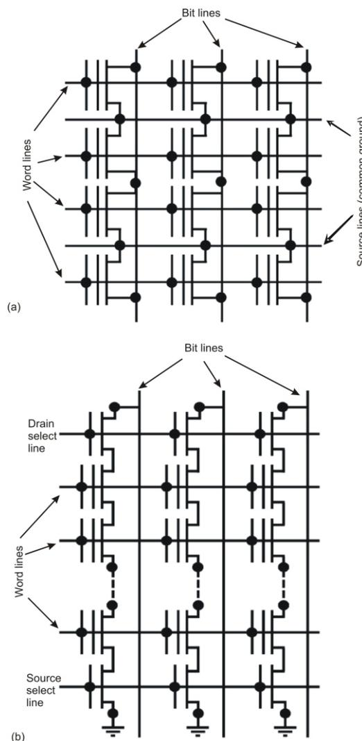
Figure 3. Flash memory cell array in (a) NOR and (b) NAND architecture
