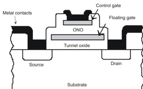
Figure 1. Lateral cross-section of a flash memory cell
