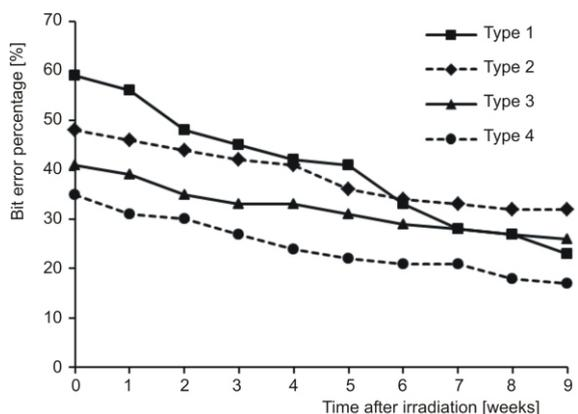
**Figure 5. Room temperature annealing of the four tested flash memory types in the nine weeks following maximum dose (12 kGy) irradiation**
