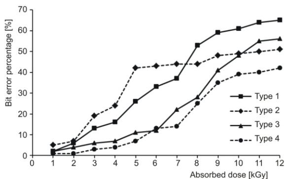
**Figure 4. Recorder values of bit error percentage vs. the absorbed dose (total ionizing dose) in the four investigated flash memory types**
