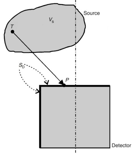
**Figure 3.** To the definition of the effective solid angle ( $\bar{\Omega}$ ), eq. (1)
