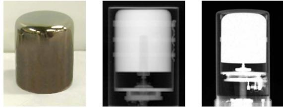
**Figure 2.** Bare HPGe crystal photograph (left), detector radiographies, showing mounted crystal inside (middle and right) [6, 7]; bulletization is clearly seen
