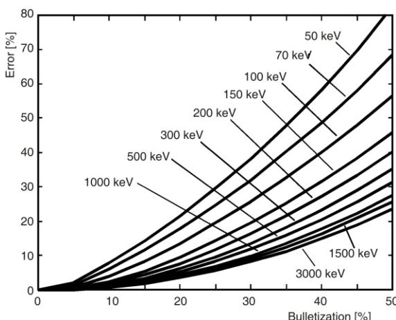
**Figure 10. Illustration of  $\delta$  vs.  $\rho/R_0$  quadratic dependence for several gamma-energies (detector: p-type HPGe 500 cm<sup>3</sup>; source: disc, 1 cm radius; source-to-detector distance: 10 cm)**
