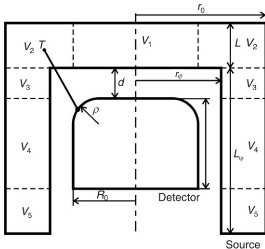
**Figure 7.** To the calculation of  $\bar{\Omega}$  for Marinelli source and bulletized detector, eq. (14)
