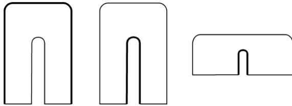
**Figure 1.** HPGe crystals with rounded edges (bulletized); thick line represents dead Ge layer; p-type HPGe (left), n-type HPGe (middle), and LEPD (right) [1]
