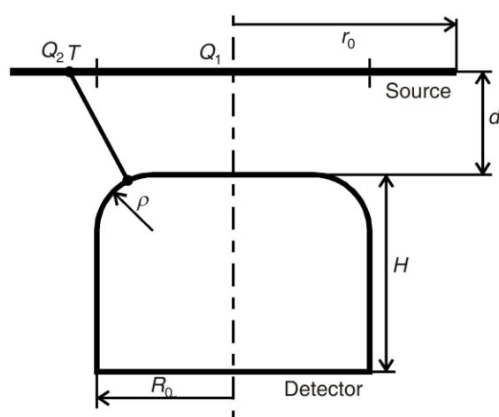
Figure 5. To the calculation of  $\bar{\Omega}$  for disc source and bulletized detector, eq. (10)
