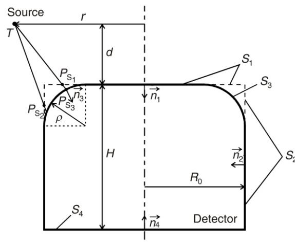
Figure 4. To the calculation of  $\overline{\Omega}$  for point source and bulletized detector, eq. (3)
