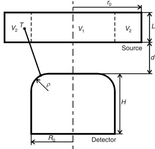
Figure 6. To the calculation of  $\bar{\Omega}$  for cylindrical source and bulletized detector, eq. (12)
