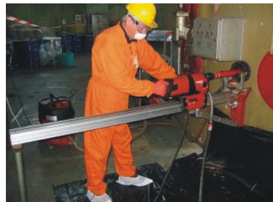
Figure 8. Sampling of the reactor block concrete by a core drilling machine
