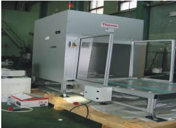
Figure 5. Gamma spectrometer with 12 plastic scintillators for free release measurements, capacity 300 kg or 1 m 3 of materials
