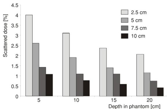
**Figure 4. Histogram plot of percent scattered dose for each depth in the phantom at various distances from the edge of the beam for field size of 5 cm x 5 cm**
