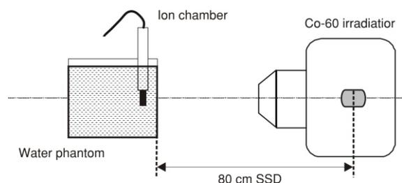
**Figure 1. Irradiation geometry for scatter dose assessment with 80 cm SSD**
