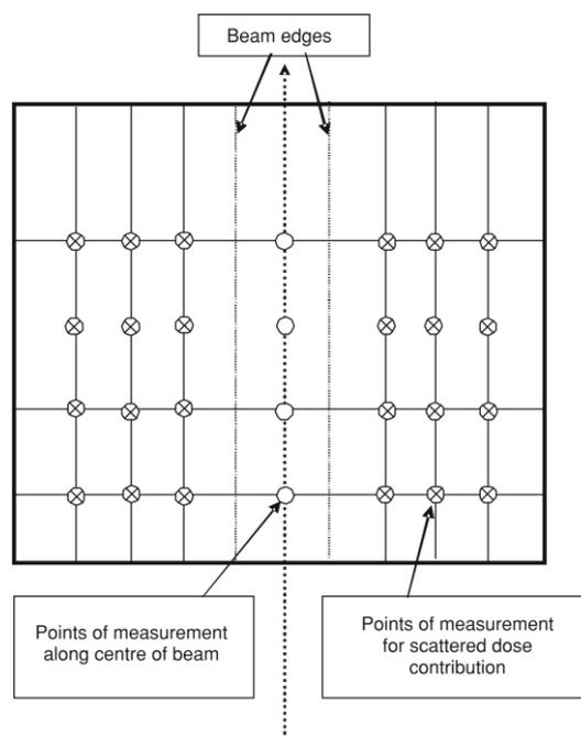
**Figure 2. Top view of PMMA water phantom showing beam edges and points of measurement**
