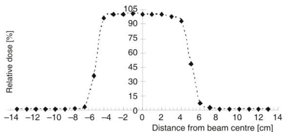
**Figure 6.** Beam profile for field size 10 cm x 10 cm at 80 cm in air to see the extent of beam penumbra
