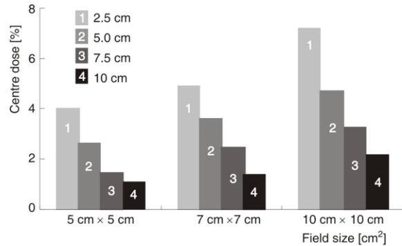
**Figure 5. Scattered radiation dose for field sizes 5 cm x 5 cm, 7 cm x 7 cm, and 10 cm x 10 cm at 5 cm depth from front wall of the phantom and for various distances from the beam edge**
