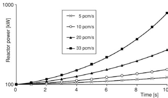
**Figure 14. Power vs. time (low power)**
