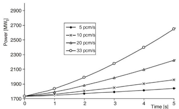
**Figure 16. Power vs. time (full power)**
