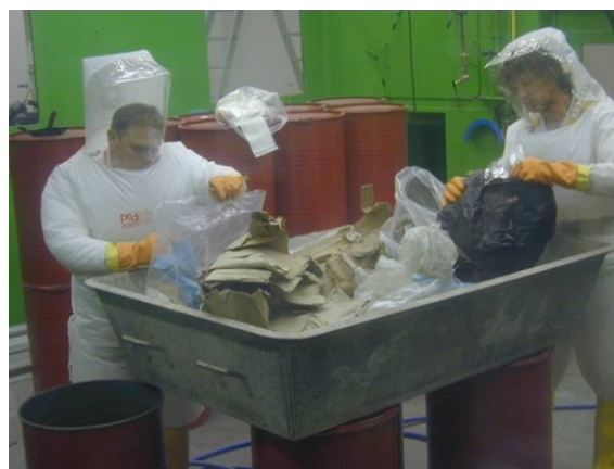
Figure 4. Waste sorting in the walk in cell
