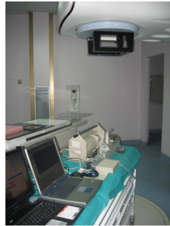
Figure 1. Experimental set-up, showing a gamma-ray spectrometer and a dose rate meter with accessories
