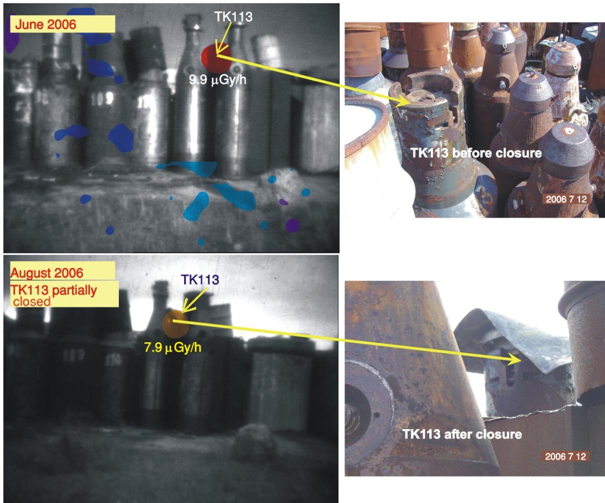
Figure 6. Composite images for the gamma-dose rates at the discrimination threshold 0.5 measured from the tripod (1 m high) installed at the central entrance at 5 m from the containers before and after TK113 closure in June-August 2006. Direction – containers 109-110
