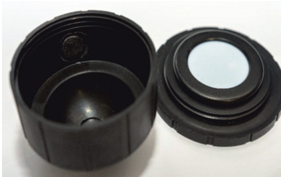
Figure 1. The EIC containing a chamber (53 cm 3 ) and an electret
