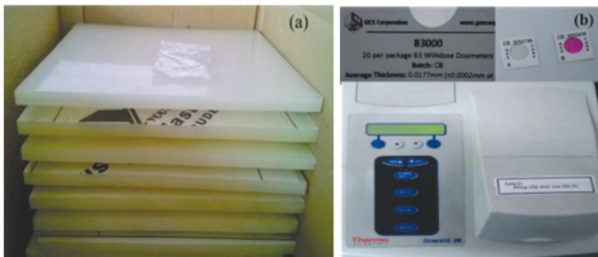
**Figure 1. The experiment of the depth – dose – profile of the electron beam from accelerator UELR-10-15S2, (a) the homogeneous dummy and (b) the film dosimeter B3000 and spectrometer GENESYS 20**
