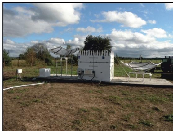
Figure 2. Measuring and monitoring SODAR/RASS system
