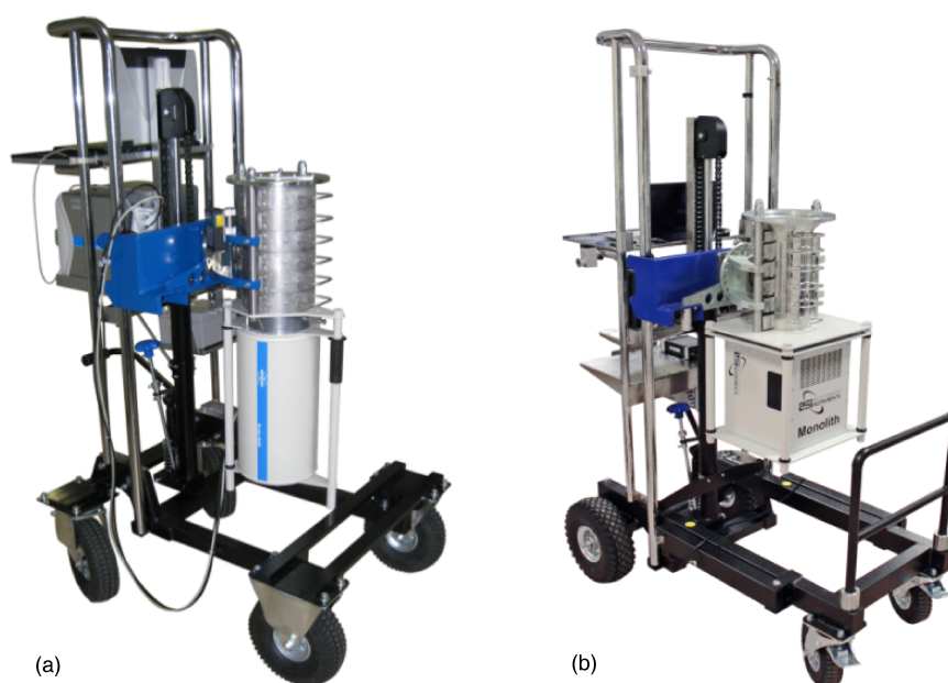
Figure1. The mobile monitor of radioactive wastes (a) with the liquid nitrogen and (b) the electromechanical cooling
