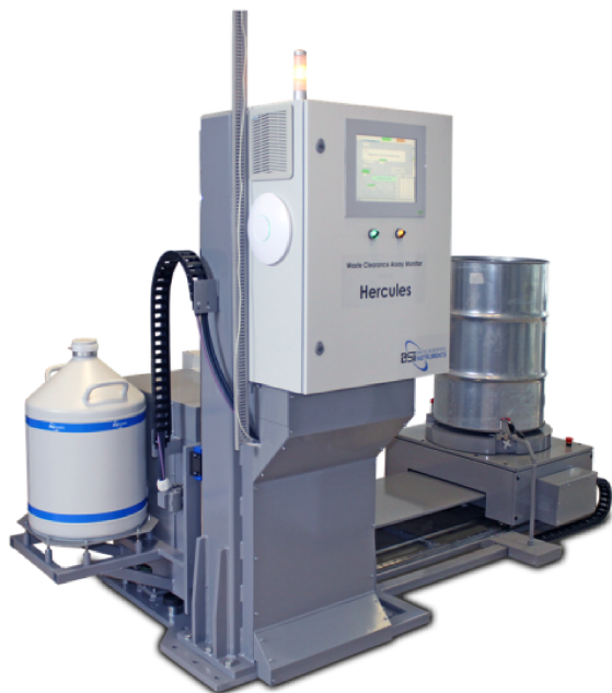
Figure 2. The Hercules 200 stationary WAM for the characterization of 200 litre barrels
