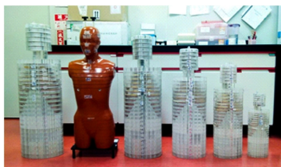
Figure 1. Use of five tissue-equivalent and Rando phantoms as patient surrogates
