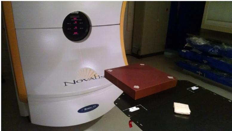
**Figure 4. Experimental measurement of the cumulative radiation dose response of Landauer nanoDots with a 6 MV X-ray source**
