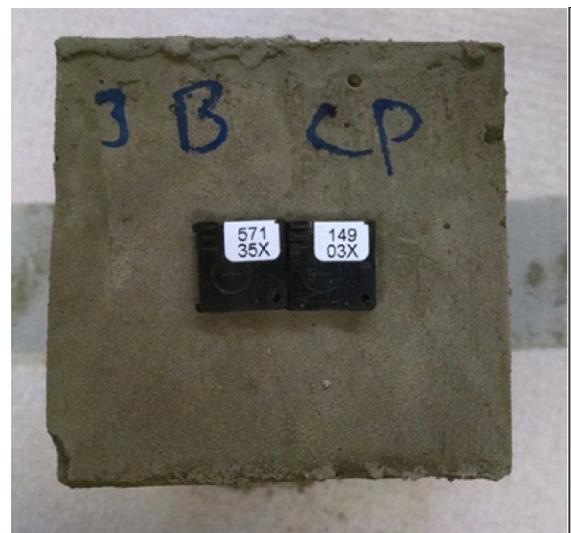
**Figure 6. Concrete cube with two nanoDots for absorbed dose measurement**
