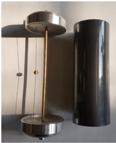
Figure 2. Photography of the GM chamber model with a conductive particle
