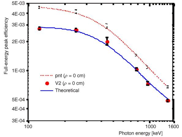
**Figure 11.** Calculated full-energy efficiency values and the measured ones, with their associated uncertainties as a function of the photon energy for the bi-detector using a (V2) mounted axial to Det-A with its centers elevated 30 cm above the common end-cap plane and a point-like source at the (V2) center
