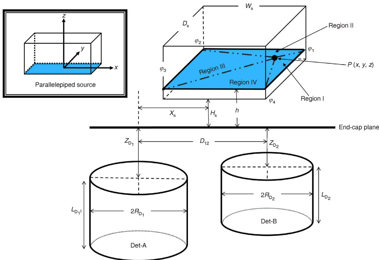
**Figure 3. Schematic diagram of the bi-detector detection system with an arbitrarily located parallelepiped source**
