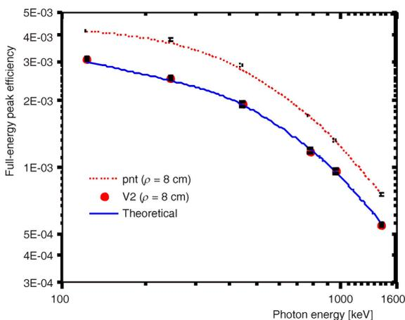
**Figure 15.** Calculated full-energy efficiency values and the measured ones, with their associated uncertainties as a function of the photon energy for the bi-detector using a (V2) mounted 8 cm lateral to Det-B with its centers elevated 30 cm above the common end-cap plane and a point-like source at the (V2)
