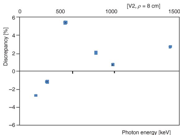
**Figure 16.** The difference percentage [%] calculated as a function of the photon energy for the bi-detector using a (V2) mounted 8 cm lateral to Det-B with its centers elevated 30 cm above the common end-cap plane
