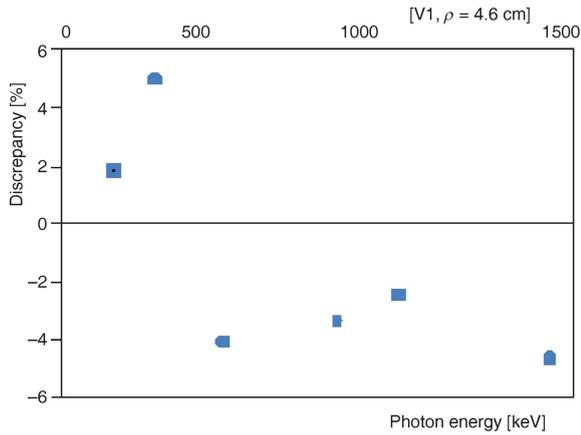
**Figure 8.** The difference percentage [ %] calculated as a function of the photon energy for the bi-detector using a (V1) mounted 4.6 cm lateral to Det-A with its centers elevated 30 cm above the common end-cap plane
