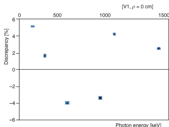
**Figure 6.** The difference percentage [%] calculated as a function of the photon energy for the bi-detector using a (V1) mounted axial to Det-A with its centers elevated 30 cm above the common end-cap
