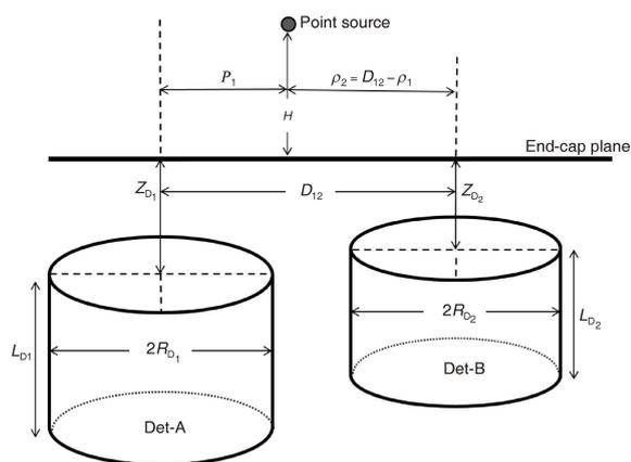
**Figure 2. Schematic diagram of the bi-detector system with an arbitrary point source**
