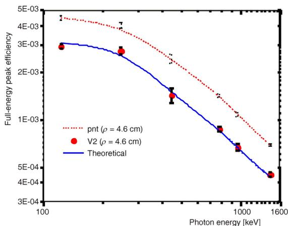
**Figure 13.** Calculated full-energy efficiency values and the measured ones, with their associated uncertainties as a function of the photon energy for the bi-detector using a (V2) mounted 4.6 cm lateral to Det-A with its centers elevated 30 cm above the common end-cap plane and a point-like source at the (V2) center
