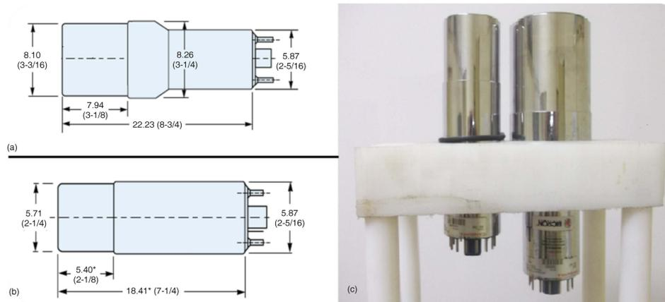
detectors mounted vertically in a specially constructed holder (fig. 4-c) made of teflon, so that the distance from side end-cap to side end-cap is 1 cm. The details of the set-up parameters of the detectors, along with acquisition electronics specifications supported by the serial and model number, are listed in tab. 4.
