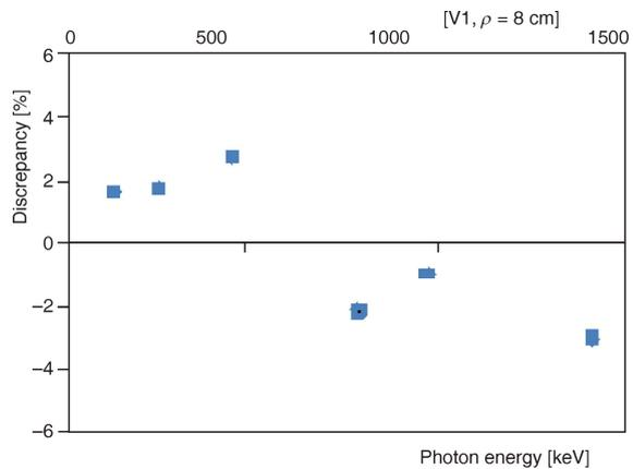
**Figure 10.** The difference percentage [ %] calculated as a function of the photon energy for the bi-detector using a (V1) mounted axial to Det-B with its centers elevated 30 cm above the common end-cap plane
