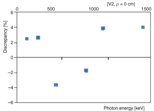
**Figure 12.** The difference percentage [ %] calculated as a function of the photon energy for the bi-detector using a (V2) mounted axial to Det-A with its centers elevated 30 cm above the common end-cap plane
