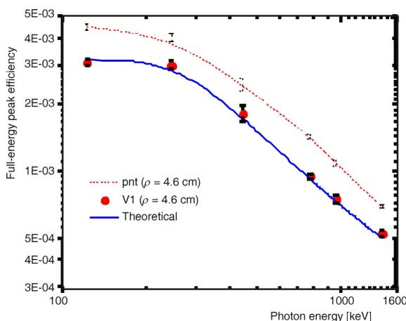
**Figure 7.** Calculated full-energy efficiency values and the measured ones, with their associated uncertainties as a function of the photon energy for the bi-detector using a (V1) mounted 4.6 cm lateral to Det-A with its centers elevated 30 cm above the common end-cap plane and a point-like source at the (V1) center
