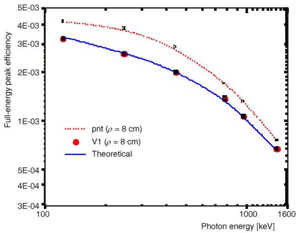
**Figure 9.** Calculated full-energy efficiency values and the measured ones, with their associated uncertainties as a function of the photon energy for the bi-detector using a (V1) mounted axial to Det-B with its centers elevated 30 cm above the common end-cap plane and a point-like source at the (V1) center
