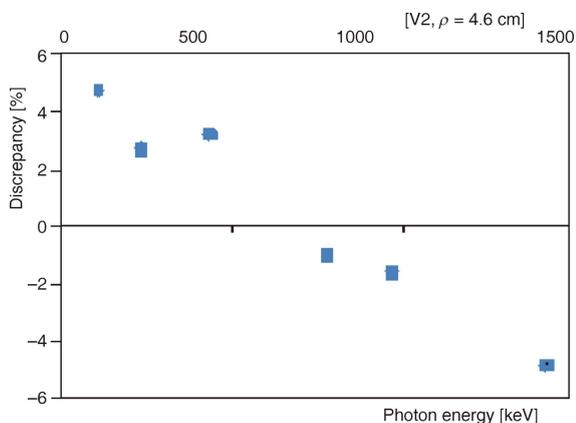
**Figure 14.** The difference percentage [%] calculated as a function of the photon energy for the bi-detector using a (V2) mounted 4.6 cm lateral to Det-A with its centers elevated 30 cm above the common end-cap plane
