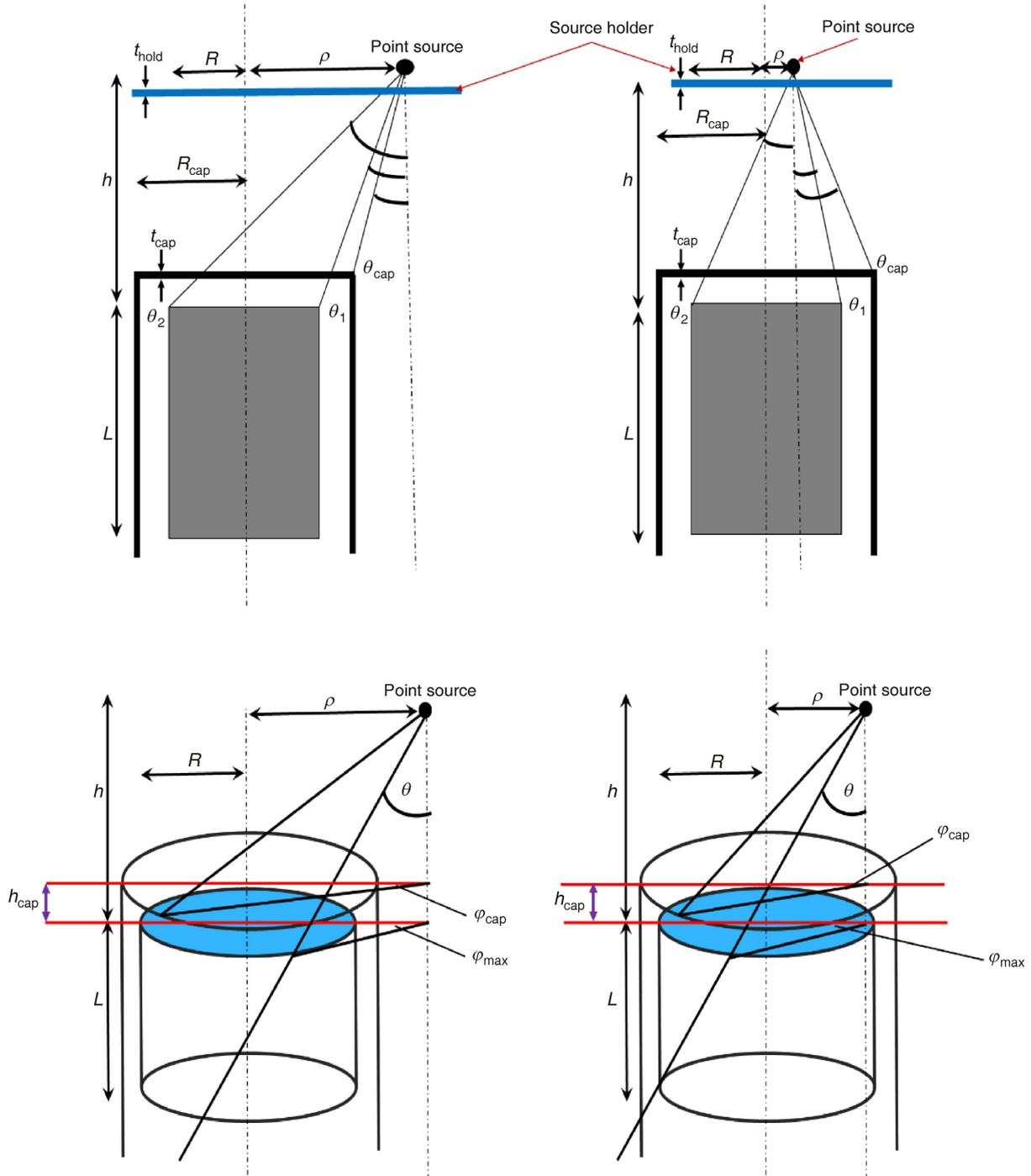
Figure 1. Arbitrarily located isotropic point source with a cylindrical detector for  $\rho > R$  and  $\rho < R$
