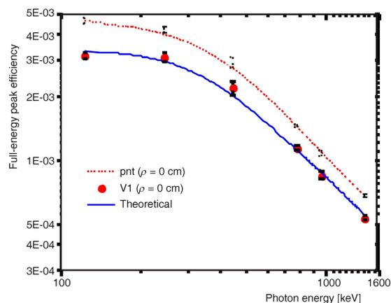
**Figure 5.** Calculated full-energy efficiency values and the measured ones with their associated uncertainties as a function of the photon energy for the bi-detector using a (V1) mounted axial to Det-A with its centers elevated 30 cm above the common end-cap plane and a point-like source at the (V1) center
