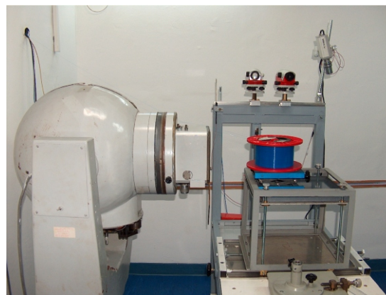
Figure 3(a). Coiled monomode optical fiber sample in front of ^{60}\text{Co} source housing
