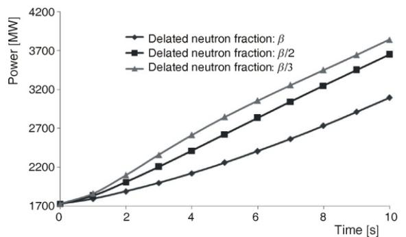
Figure 7. Effect of delayed neutron fraction ( $\beta$ ) at high power
