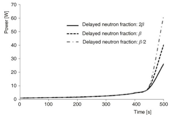
Figure 1. Effect of delayed neutron fraction in subcritical phase of kinetics
