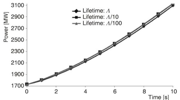
Figure 6. Effect of neutron lifetime ( $\lambda$ ) at high power
