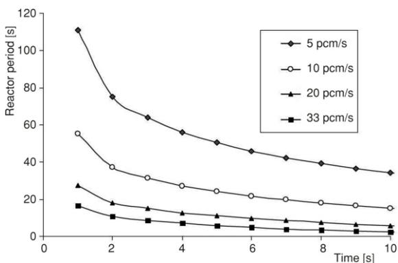
**Figure 15. Reactor period vs. time (low power)**
