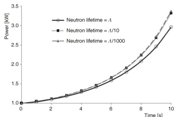
Figure 2. Effect of neutron lifetime at low power
