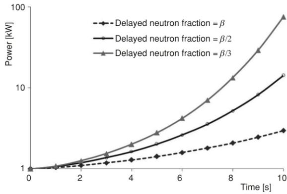
Figure 3. Effect of delayed neutron fraction at low power
