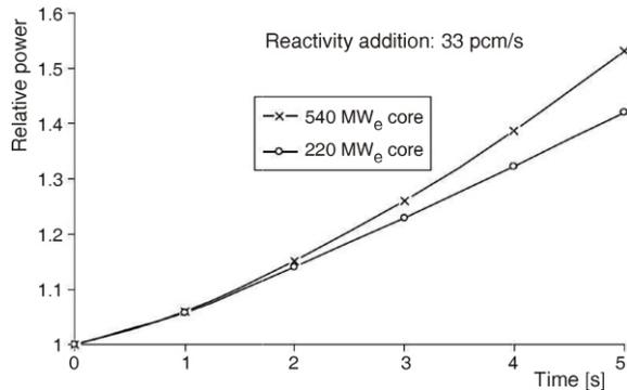
Figure 11. Core size effect (high power)
