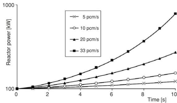
**Figure 14. Power vs. time (low power)**
