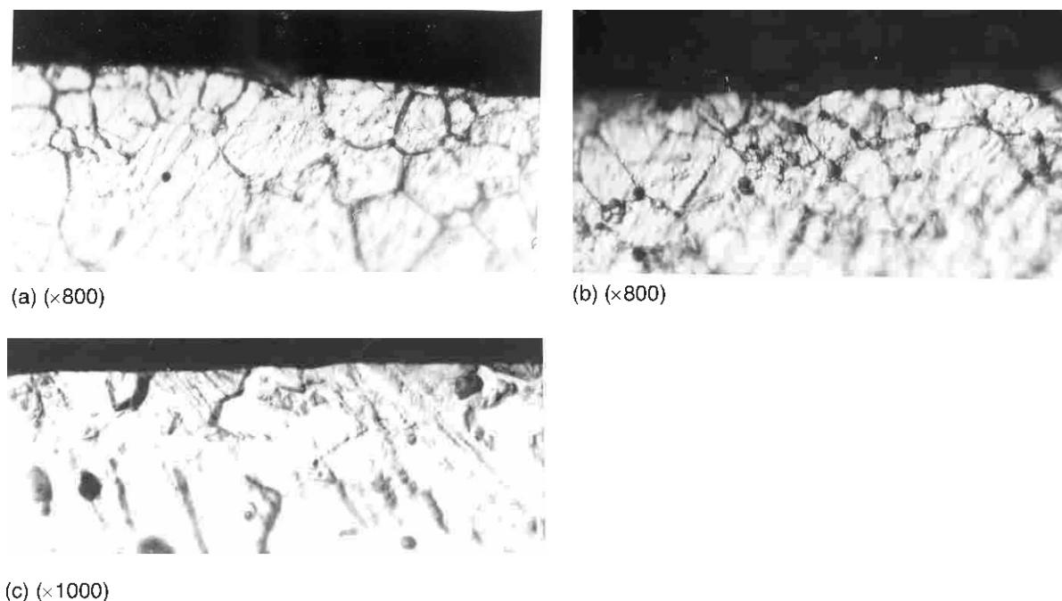
**Figure 9.** Microcracks initiated at the surface of the sample stressed at 490 MPa tested 48 hours at 85 °C at following potentials: (a) -100 mV, (b) -157 mV, and (c) +80 mV
