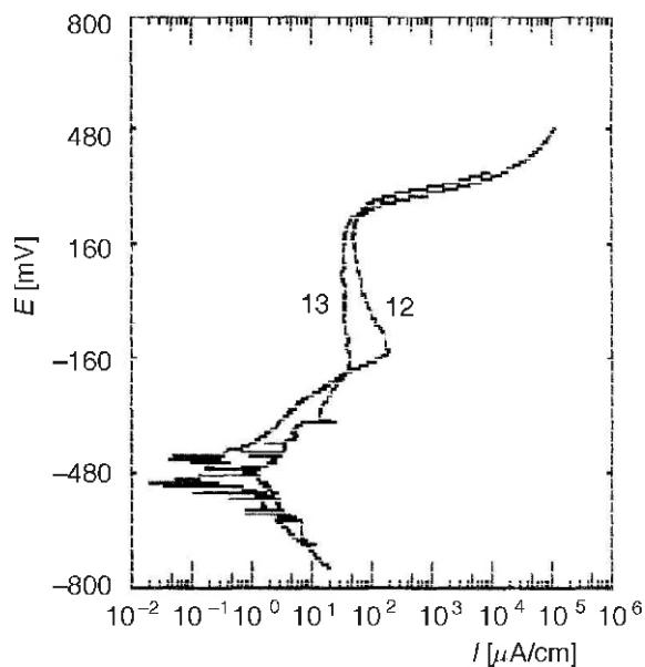
Figure 7. The PD curves for the unstressed sample (curve 13) and stressed sample (curve 12) at 85 °C
