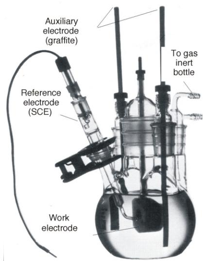
Figure 4. Electrochemical cell [6]
