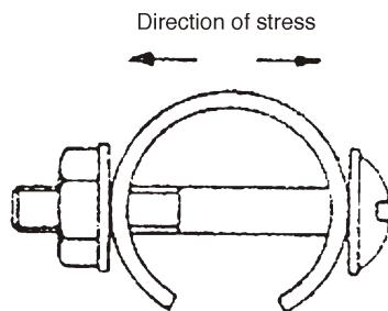
**Figure 1. The C-ring to test the susceptibility of Incoloy-800 to SCC (external diameter 15.9 mm, height 12 mm)**
