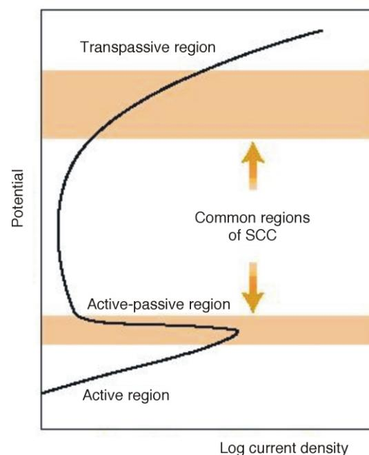
Figure 5. The effect of potential to SCC susceptibility [7]
