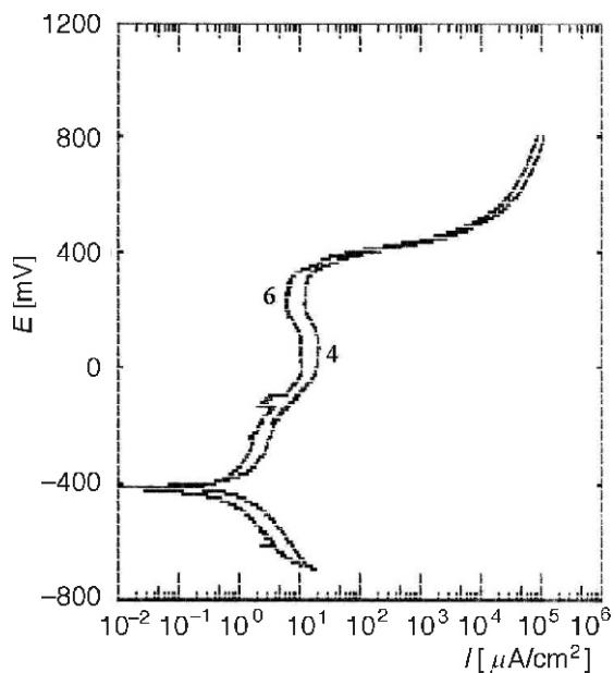
Figure 6. The PD curves for the unstressed sample (curve 6) and stressed sample (curve 4) at room temperature
