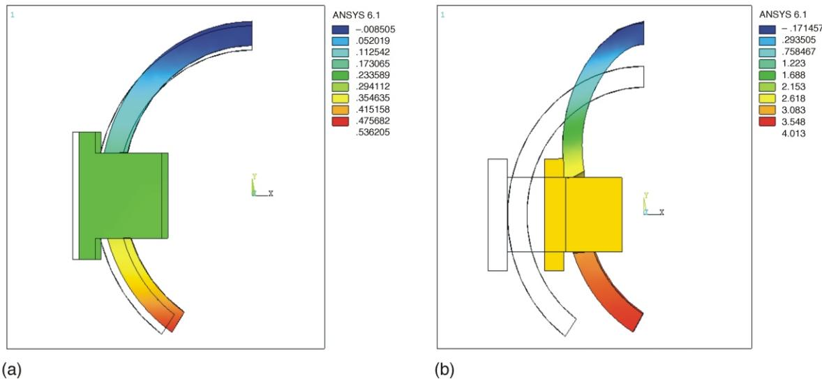
**Figure 2.** The displacement of the ring in the x direction
