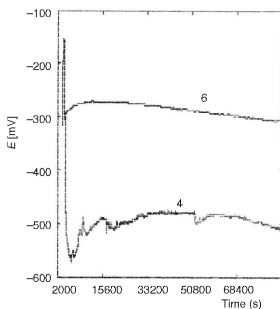
Figure 8.  $E_{corr}$ -time curves of the unstressed sample (curve 6) and respective stressed sample (curve 4) tested for 24 hours at 25 °C
