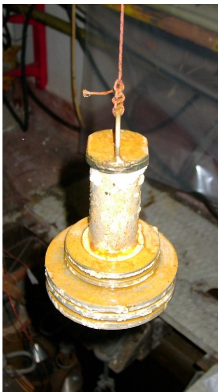
Figure 30. Rack#2.2/CRP-I after 24 months of exposition time
