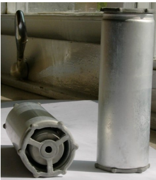
Figure 2. TVR-S fuel element
