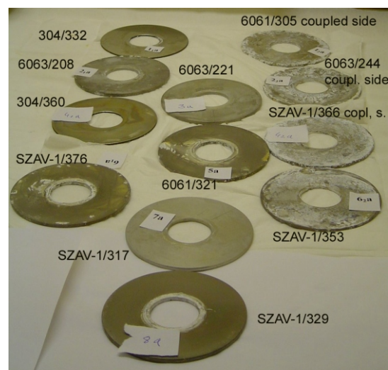
Figure 39. Front side (A) of coupons of disassembled Rack#2/CRP-II
