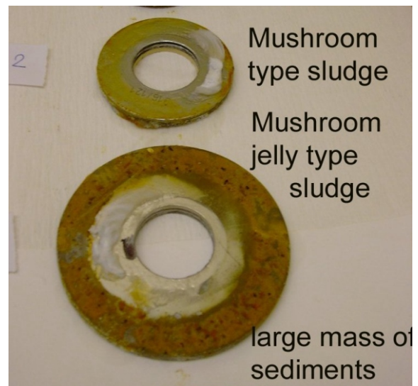
Figure 18. Mushroom-jelly type of sludge and red-brown deposits at the front side (A) of 6063/159 (lower one) and 316/121 coupon
