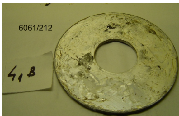
Figure 34. Crevice corrosion at the coupled side of coupon 6061/212
