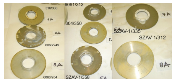
Figure 23. Front side (A) of coupons of disassembled Rack#1/CRP-II
