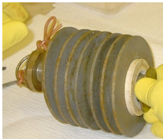
Figure 8. No sediments at the back side of coupons of Rack#1/CRP-I
