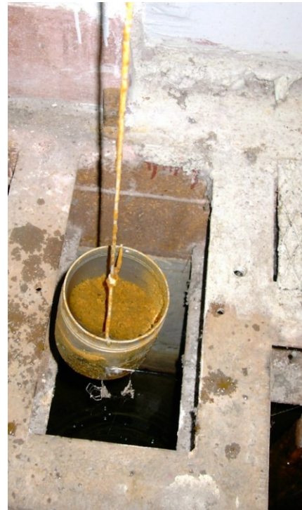
Figure 5. Withdrawn of the pot used for sludge sedimentation from the pool
